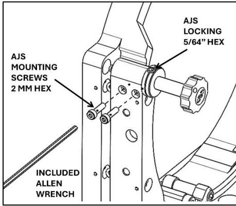
The included 2 mm (5/64") Allen wrench secures the AJS mounting screws and can also be used to engage the AJS flexure lock.
