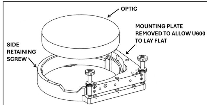
**STEP 3:** Re-install the brackets and finger-tighten the Optic Retaining Set Screws with included 3 mm Thumb Hex Tool.
