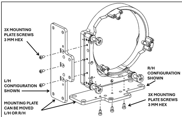
To switch between left-hand and right-hand configurations, the mounting plate must be repositioned. The figure shows the location of the three screws that need to be removed to make this change (3 mm Allen included with U600-AC model). The plate also needs to be removed when swapping out AJS adjusters.
