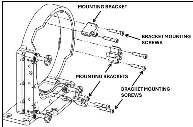
**STEP 2:** With the brackets removed, insert the optic and hold in place with the Side Retaining Set Screw (finger-tight only). If possible, this process should be done horizontally to make optic handling easier.
