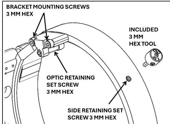
The included 3 mm hex tool fits the optic retaining soft-tip set screws, the side optic retaining screw, and the bracket mounting screws.
